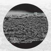
SEM picture of Mem-Lok® Pliable at 50-fold magnification – not side-specific; dense, uniform single layer
